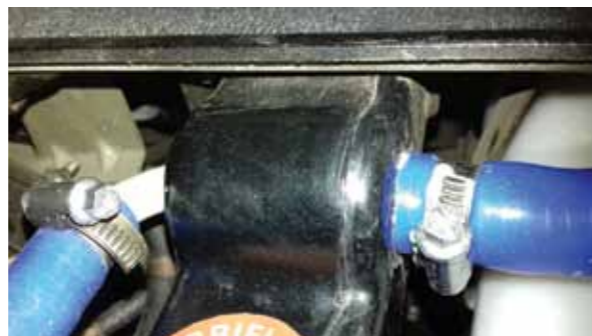
Fan housing for the coolant cooler
