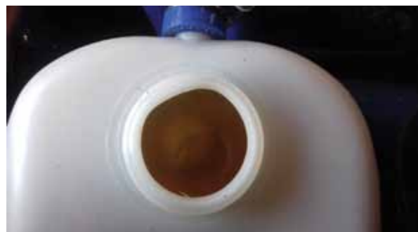
Deformed filler mouth on expansion bottle
