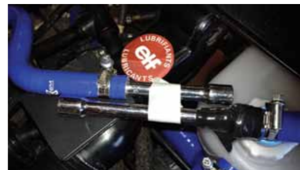
Get me home solution, by bypassing the cooler
