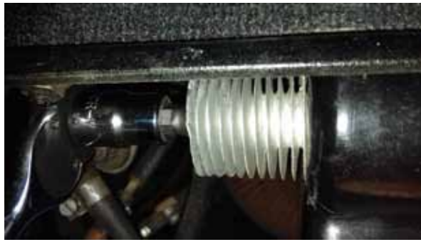
Screwing in the finned cooler section
