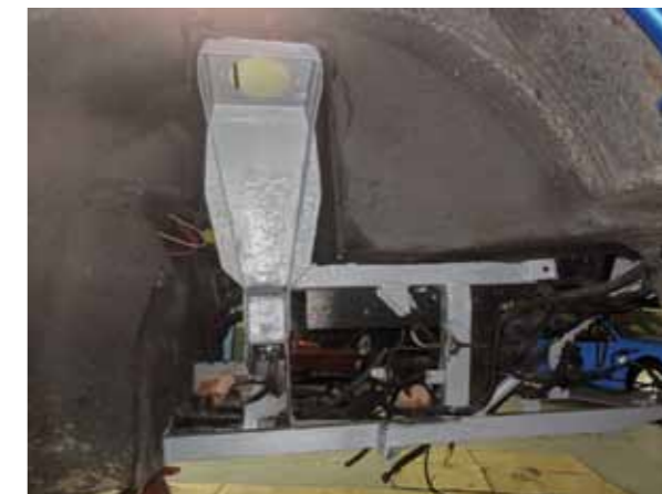
Repaired sub frame parts
